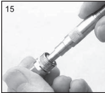
15. Fit Seal to Housing (10).
