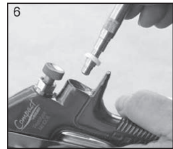
6. Remove Valve Seat.
