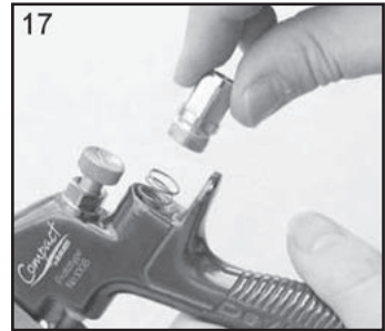
17. Replace Valve Spring and screw in Housing (10).
