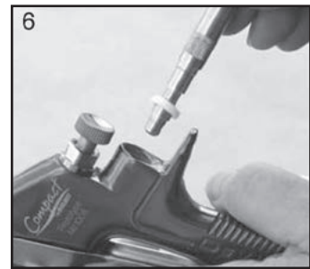
6. Remove Valve Seat.
