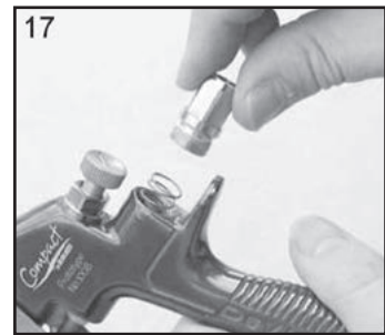
17. Replace Valve Spring and screw in Housing (10).
