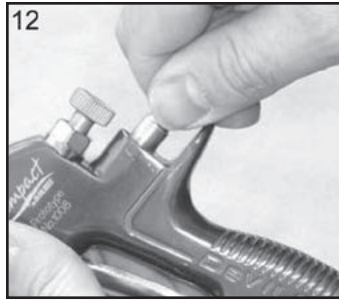
12. Fit Valve Seat to Gunbody.
