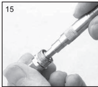
15. Fit Seal to Housing (10).
