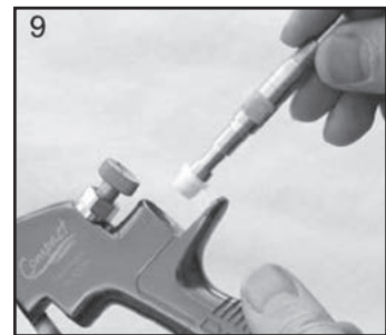
9. Fit New Front Seal to Service Tool.
